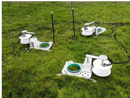
Monitoring CO 2 fluxes in experiments investigating impacts of CO 2 leaks on agricultural soils and crops
